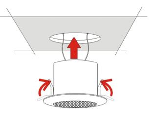
(4) Push back wire clips and slide speaker into place.
