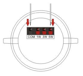
(2) Check cables are correctly connected. COM & 5W
